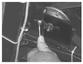
Step 1. Loosen Belt Tensioning Nuts.
